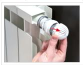
**1)** Turn the knob to position (3) and release it by pulling it forward.
