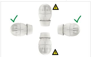
⚠ These positions are not recommended due to the influence of the radiator temperature on the thermostatic head.
